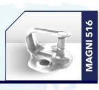
Magni 516 is a chrome-free hybrid coating that combines electroplated zinc/nickel and hex-chrome-free passivated substrate with an aluminum-rich organic topcoat. A coating that can be engineered to specific coefficient-of-friction needs, Magni 516 is offered with exempt solvents and typically applied to fasteners, including nuts, bolts and other hardware. Magni 516 can be applied via dip-spin or spray application methods.
