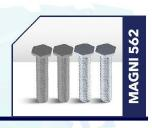
Magni 562 is a chrome-free duplex coating that combines electroplated zinc nickle and hex-chrome-free passivated substrate with an aluminum-rich organic topcoat. A coating that can be engineered to specific coefficient-of-friction needs, Magni 562 is offered with exempt solvents and typically applied to fasteners, including nuts, bolts and other hardware. Magni 562 can be applied via dip-spin or spray application methods.
