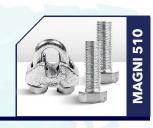
Magni 510 is a chrome-free duplex corrosion protection coating that combines electroplated zinc and hex-chrome-free passivation with a chrome-free aluminum-rich organic topcoat. Engineered for use on fasteners, Magni 510 is typically applied to nuts, bolts, screws and other hardware.
