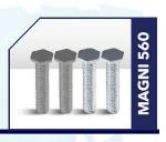
Magni 560 is a chrome-free duplex coating that combines electroplated zinc and hexchrome-free passivated substrate with an aluminum-rich organic topcoat. A coating that can be engineered to specific coefficient-of-friction needs, Magni 560 is offered with exempt solvents and typically applied to fasteners, including nuts, bolts and other hardware. Magni 560 can be applied via dip-spin or spray application methods.
